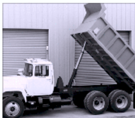
Telescopic head hoist—NTEA Type IV—Class 80 thru 110—cast iron hydraulic pump. All hydraulics made in USA.
